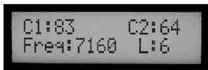
A front-panel LCD "turns counter" shows the capacitor and inductor settings, as well as the operating frequency.
